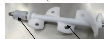
Fig. A Bellows type sealing ring + stirrer
